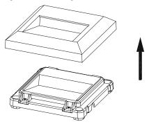
Undo the 4 cover fixing screws and remove the clear plastic cover.
