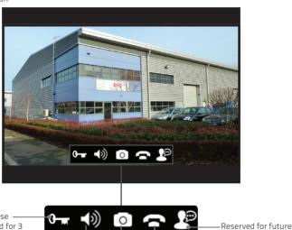
Lock release Press and hold for 3 seconds to activate doorstation lock output
