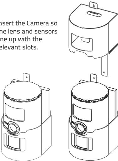
4. Using the security screws provided, secure the two tabs together.
