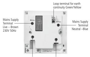
Switched Live Terminal Load live connection – Brown Switched Neutral Terminal Load Neutral connection – Blue
