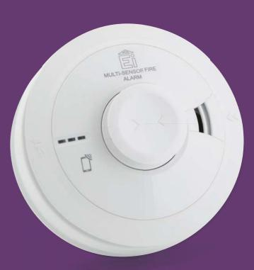
The alarm provides total coverage to all fire types by actively monitoring both sensors. If a temperature rise is detected, the intelligent alarm software increases its sensitivity to smoke, detecting the fire quicker and more accurately.
